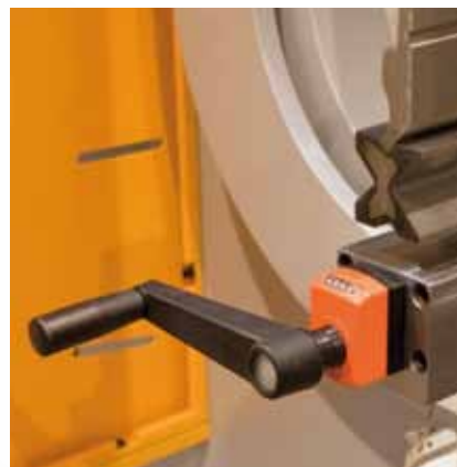
Manual Crowning System (*) Manual crowning system that enables the part to be at even bending angle at any given point.
